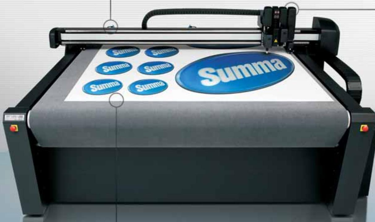
The **Tangential module** is the most powerful and most flexible module: it offers a vertical force of 12 kg and corresponds to a whole range of matching tools. Each tool has its own barcode ID that ensures automatic recognition and parameter setting.
